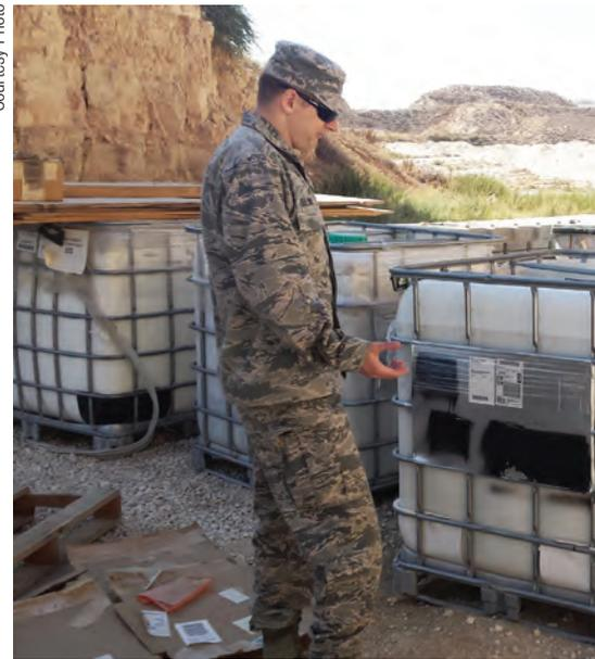
**An Army and an Air Force engineer review a pallet of containers of DLA-provided ground-hardening paste, commonly called "rhino snot," which is used to reduce dust. This shipment was used to coat a makeshift runway for an unmanned aerial system.**
